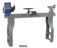
Model No. Mfg. No. KWL-1443VS 14 1/2" Swina: Distance between centres: 43" MT #2 Headstock and tailstock taper: Spindle size: 1" x 8 TPI Spindle bore: 3/8" Speeds: 600-2400 RPM Motor: 6.6 A, 1 phase, 60 Hz Voltage: 110 V **Dimensions:** 62" L x 14 1/2" W x 48" H Weight: 310 lbs. Price/Each Ś
