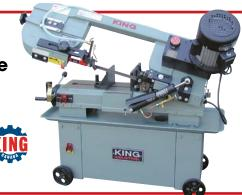
Model No. BV709 Mfg. No. KC-712GH-5 Cutting capacity at 90°: Rect. 7" x 12", Round 7" Cutting capacity at 45°: Rect. 4-1/2" x 5", Round 5" 3 (110, 230, 340 FPM) Speeds: Blade: 0.75" x 0.032" x 93" Motor: 1 HP, 14 A, 1 phase, 60 Hz Voltage: 110 V Dimensions: 47" L x 21" W x 40" H
