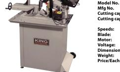
KC-129DS Mfg No. Cutting capacity at 90°: Rect. 5" x 6", Round 5" Cutting capacity at 45°: Rect. 4" x 2 15/16"; Round 5" Speeds: 3 (80, 120, 200 FPM) Blade: 64-1/2" x 1/2" x 0.25" Motor: 6 Amps Voltage: 110 V, 1 phase, 60 Hz 39"L x 23" W x 43" H **Dimensions:** Weight: 180 lbs.
