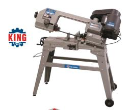
Model No. **UAJ228** Mfa. No. KC-129C Cutting capacity at 90°: Rect. 4-1/2" x 6" Round 5" Cutting capacity at 45°: Rect. 3" x 4-1/2" Round 3" 3 (80, 120, 200 FPM) Speeds: Blade: 64-1/2" x 1/2" x 0.025" Motor: 8 A, 1 phase, 60 Hz Voltage: 115 V
