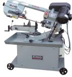
**TBU410** Model No. Mfg. No. KC-712DS Cutting capacity at 90°: Rect. 7" x 12", Round 7" Rect. 3-1/2" x 5-1/2", Round 5" Cutting capacity at 45°: Speeds: 4 (98, 164, 246, 328 FPM) 0.75" x 0.032" x 93" Blade: 1 HP, 6.2 A, 1 phase, 60 Hz Motor: Voltage: 220 V **Dimensions:** 50" L x 26" W x 44" H 325 lbs. Weight: Price/Each
